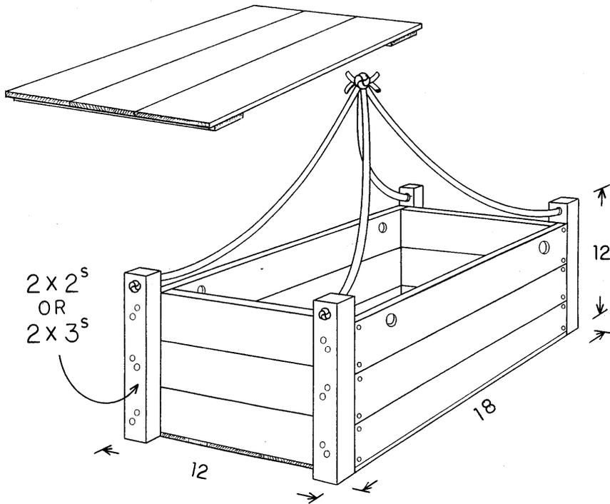
Figure 15. Stackable crate for large items or sprouting
