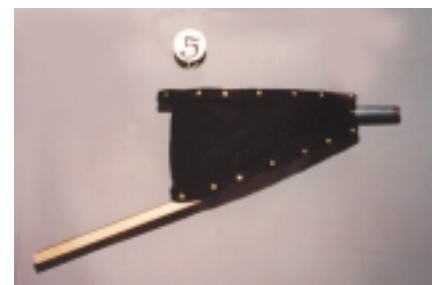
Photograph #5. The completed bellows
