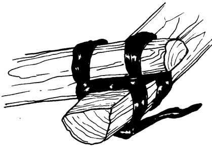
Figure 2. A notched and lashed joint.
